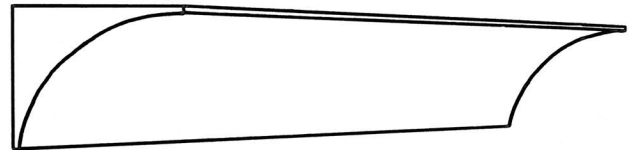
CP117 Projection 228mm(9") Depth 228mm(9")
