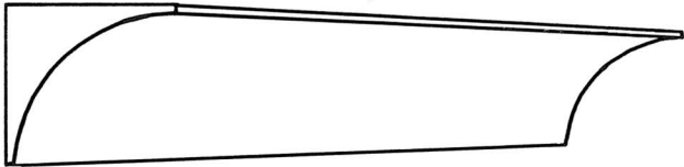
CP122 Projection 140mm(5 1 / 2 "") Depth 140mm(5 1 / 2 "")
