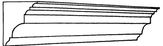
CP57 Projection 80mm(3 1/8") Depth 90mm(3 1/2")
