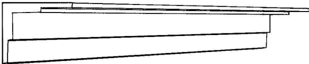
CP214 Projection 102mm(4") Depth 90mm(3 1 / 2 " )
