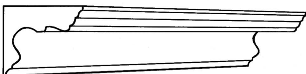
CP88 Projection 134mm(5 3/8") Depth 120mm(4 3/4")
